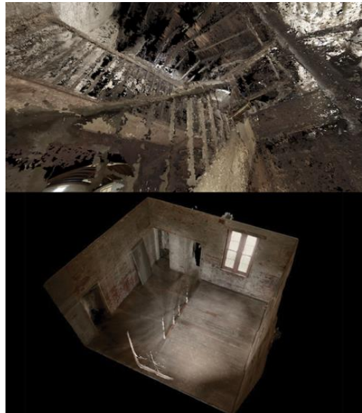
Figure 6, 7: Point-cloud representation, captured with action camera rig (t). Textured mesh of interior spaces, captured with a DSLR (b).
