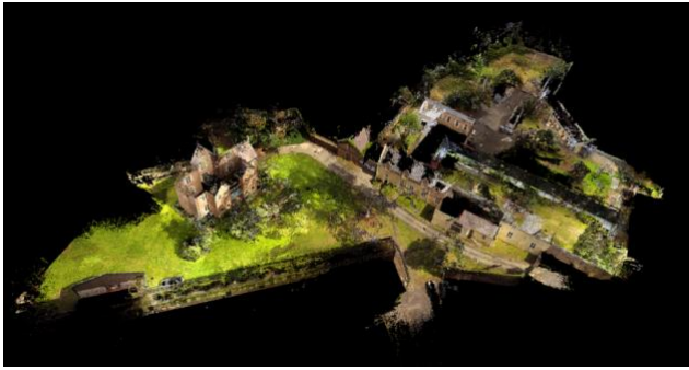
Figure 13, 14: Aerial view point-cloud representation of the site in Parramatta, 1.5ha, 24M points (l). Point-cloud representation close-up (r).
