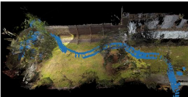
Figure 8: Photogrammetry processing terrestrial survey. The photographs of the camera cluster are represented as blue quads ( Agisoft Photoscan ).
